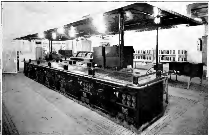
Close-up of the Edison range in first class galley.
